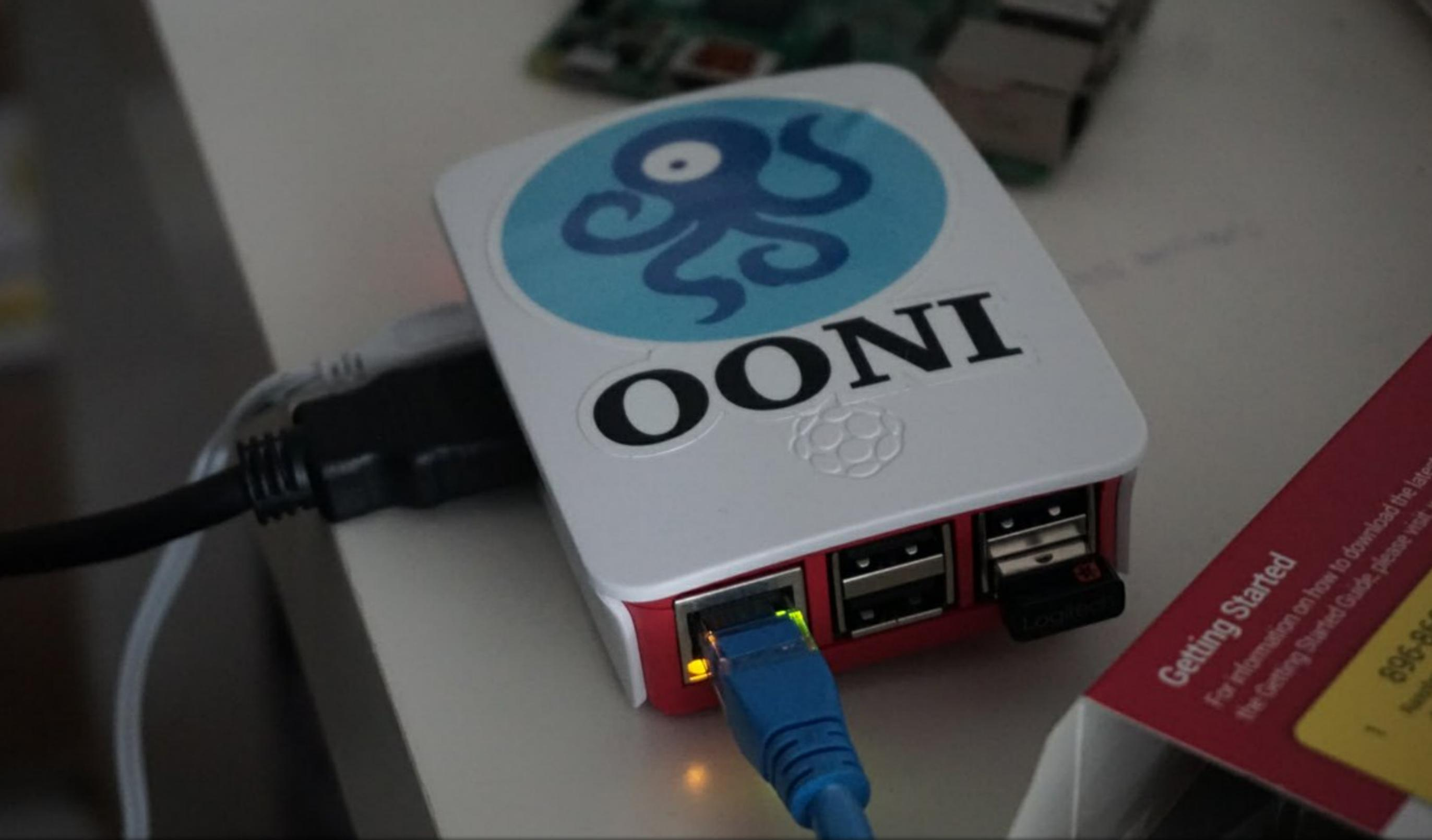
ooniprobe on RaspberryPi
